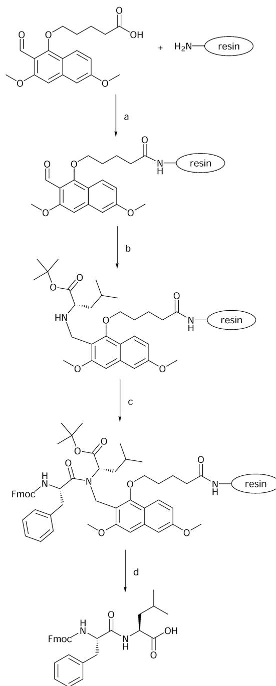
**Scheme 3** Solid-phase synthesis of Fmoc-Phe-Leu-OH on NAL-3. Reagents and conditions: (a) HBTU-DIEA-HOBt-DMF, 16 h, rt, then 30% Ac<sub>2</sub>O, DMF-DIEA (catalytic amount), 3 h, rt; (b) H-Leu-OtBu-HCl-NaBH<sub>3</sub>CN-DMF, 16 h, rt; (c) Fmoc-Phe-OH-DIPCPI, CH<sub>2</sub>Cl<sub>2</sub>-DMF 9 : 1, 16 h, rt; (d) acidolytic release from NAL-3 resin, see Table 1.
